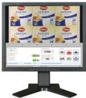
Display on Touch-screen HMI
