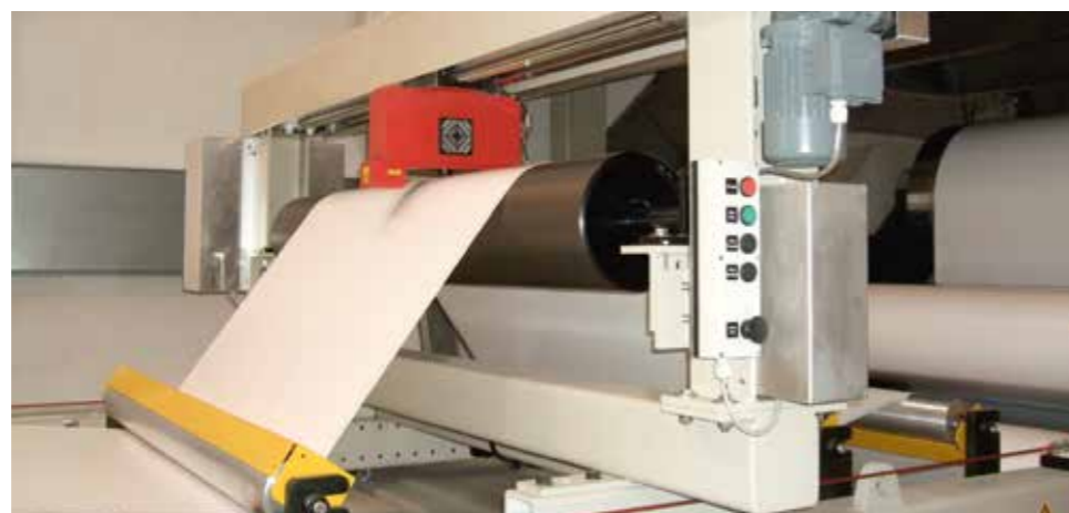
Measuring system with an optical thickness sensor ,Shadex'
