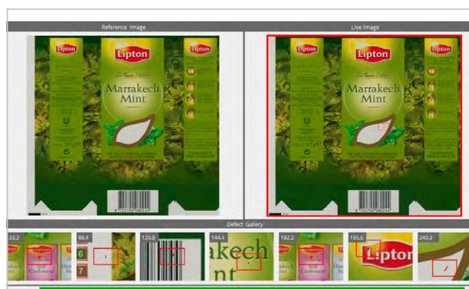
In the defect gallery, the last defects can be conveniently displayed and selected.
